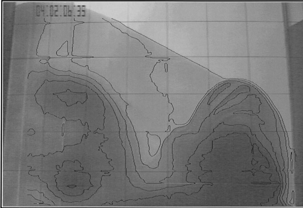
FIGURE 7. A processed image from an experiment (run 26: rotation rate = 6 s/rev, Q = 27 \text{ cm}^3 \text{ s}^{-1} , D = 8.5 \text{ cm} ) with the thickness of the flow estimated from the image intensity. The contours are at intervals of approximately 1.1 mm. In this experiment the downslope flow is strongly modulated by the instabilities, with very little flow in between them. Downslope of the right-hand dome/eddy there is a suggestion of two or three short wave crests in the draining flow. However, the draining flow downslope of the left-hand eddy is concentrated in a single feature that is nearly as thick as the dome.
